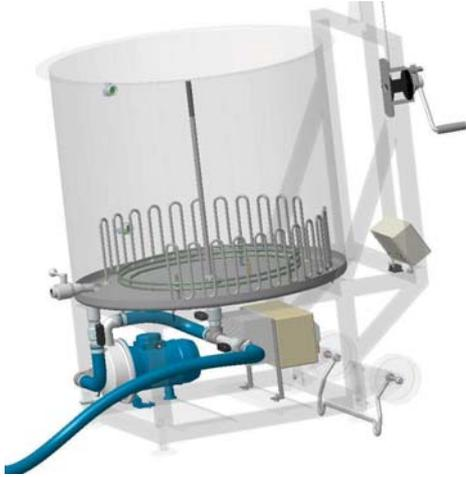
Place the Braumeister in the cleaning position by folding down the rear supporting bracket which holds the Braumeister inclined. Connect the hose to the waste water system and position the valves as per the figure on the left. Now you can clean the Braumeister from above with a suitable brush and water and at the same time pump the waste water (in manual mode) into the drain.
