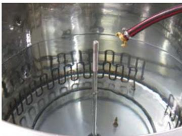
Fill up the kettle with 230 l brewing water – up to the top mark on the drawbar or alternatively on the filling level sensor. Follow the instructions on the brewing control, by acknowledging with ENTER that water has been added. The pump primes itself and the programmed mashing temperature is started.
