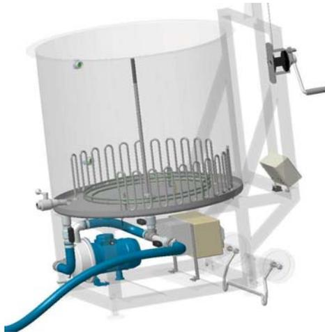
Immediately after brewing, it is best to place the Braumeister in the cleaning position (see figure, left) and to pump off all the fine solids diluted with water. Observe the correct valve positions.
