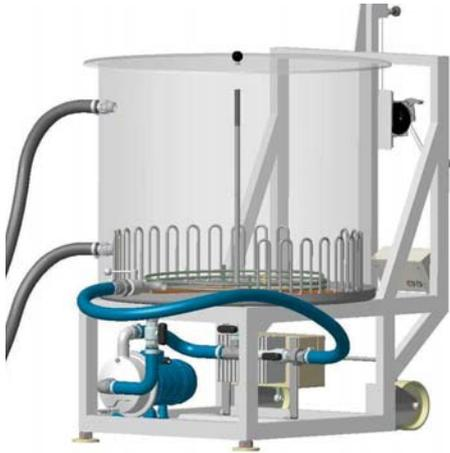
To do this, connect up the hoses and position the valves as per the figure on the left. With a low pump speed (dial position 6-8) you achieve a smooth rotation of the wort in the kettle. Caution!: the pump only switches back on at 86°C. In addition, the rotation helps to optimise cooling. In this case, a cooling time of roughly 50 mins. is required to go from 100°C down to 20°C.
