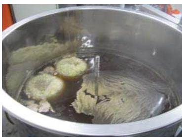
Continue with START, to start boiling the hops. Do not put the lid on. Avoid boilover. Add the first hops (200g) 10 mins. after start of boiling. Do not put the lid on even when boiling the hops. Vapours must be able to escape. Top up the evaporated water or adjust the original gravity. The last hop addition (100g) takes place 10 mins. before flame out.
