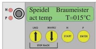
Plug in the Braumeister. The control system is then in start mode. To program a recipe and its time and temperature parameters, press the ENTER key for 1 sec.
