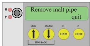
After removing the malt pipe, acknowledge this with ENTER. To start the hop boiling, press START. The pump and heating are switched on and the automatic process continues.
