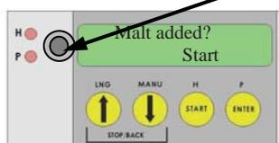
When you have added the malt, acknowledge with ENTER. For safety's sake, the question is repeated "Malt added?". By pressing START, you now start the actual brewing process with the Braumeister. The pump and heating switch on. The wort rises in the pipe and runs over. The cycle has started and during the next phases the important elements are extracted from the malt by the circulating wort.
