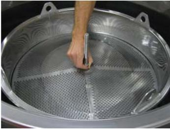
Once the mashing temperature is reached, a warning tone sounds which you acknowledge with ENTER. Now insert the malt pipe (with seal fitted, facing downwards). Take care that the seal and the malt pipe are centred and are sitting absolutely level on the kettle bottom. Insert the first sieve right down to its lower rim.
