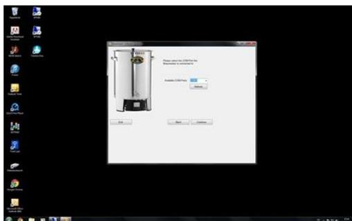
Connect the module (port on the side of the module) to your PC using the USB cable. Wait until your operating system automatically finds a suitable driver and installs it. You should then connect the Braumeister to the mains. Launch the *software updater* and transfer the latest firmware (hex file) to the controller. Unplug the Braumeister and remove the USB cable. The latest version should now be on the controller.
