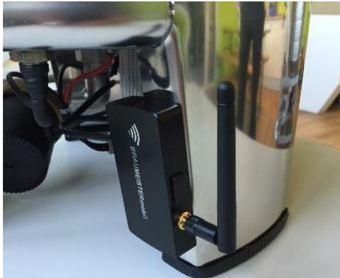
Remove the WLAN module from the protective carton and mount it on a Braumeister base. Plug the cable gland into the free socket on the reverse side of the Braumeister controller and tighten (connect the temperature sensor as well).
