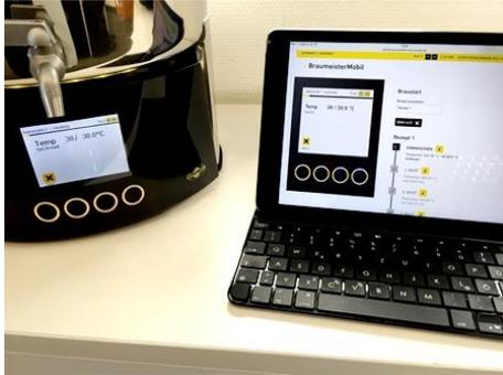
Entering the IP address into the browser address line calls up the monitoring software over the Internet and, with some delay, loads the data from the controller.
