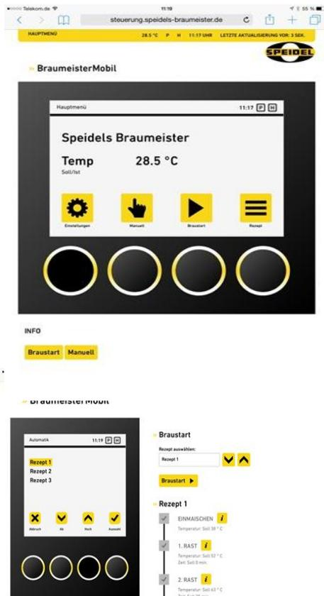
An image of the Braumeister controller is displayed. You can intervene in a controlled manner by starting a recipe, or manually, by turning the heater and pump on/off. Making settings, processing recipes and selecting temperatures needs to be performed manually on the device. In an emergency, the programme can also be stopped and terminated online.
